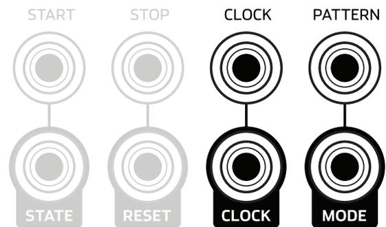
The PATTERN output combines the step outputs into a single pulse stream. The GATE/TRIG switch controls the duration of the PATTERN output pulses.
